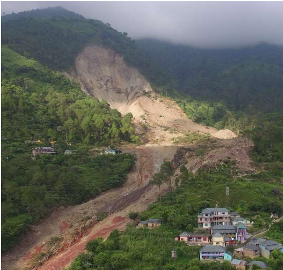
Fig. 1. (Left) Water triggered Paddhar landslide in 2017 in Himachal Pradesh due to intense and persistent rainfall. The failed slope was approximately 250 m high and 150 m in width. Approximately 300 000 m 3 debris was displaced for approximately 950 meters resulting taking 46 lives. (Courtesy: Himachal Pradesh State Disaster Management Authority)
