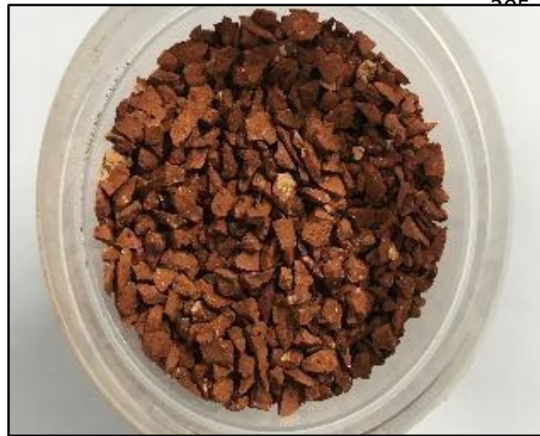
Fig. 9. A view of the rubble brick used for model earthquake drains
