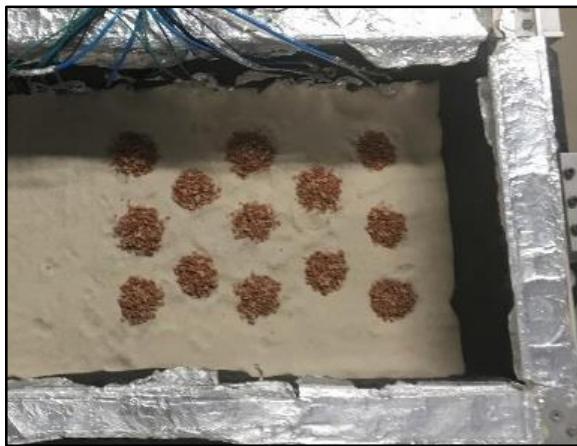
Fig. 11. Plan view of the rubble brick drains in Hostun sand in the laminar container
