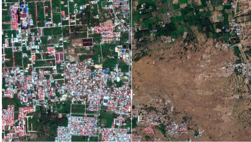
Fig. 2. Pre and Post-earthquake satellite images of the destruction due to lateral spreading
