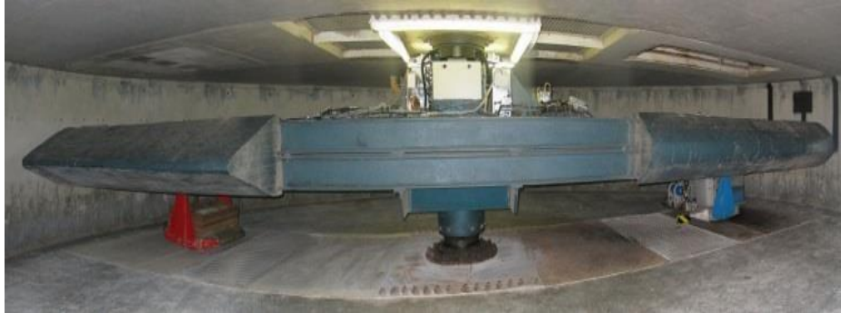
Fig. 5. A view of the 10 m diameter Turner Beam Centrifuge
