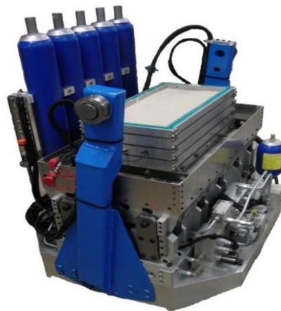
Fig. 6. A view of the servo-hydraulic earthquake actuator
