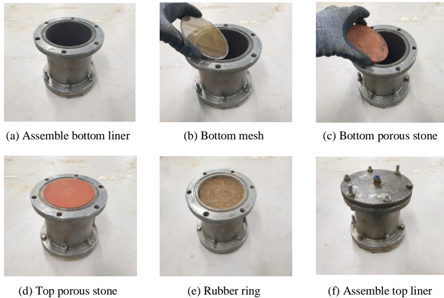
Fig. 4. Test procedures of permeability test for recycled soil specimen
