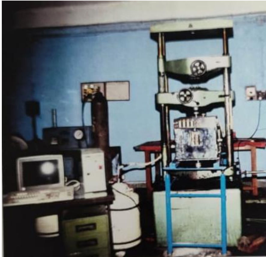
Fig.1 (a) - Laboratory testing of rocks at sub-zero temperature
