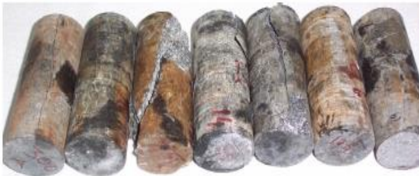
Fig. 9 - Fracture pattern in charnockite rock specimens after UCS test
