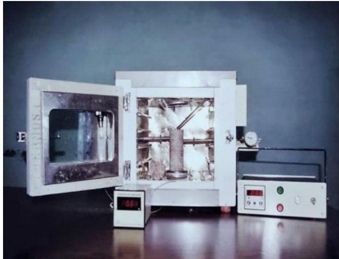
Fig.4 - Inside view of Environmental chamber for heating during rock testing
