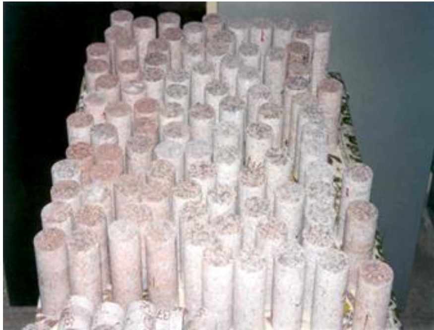
Fig. 8 - Granite specimens ready for testing under high temperature
