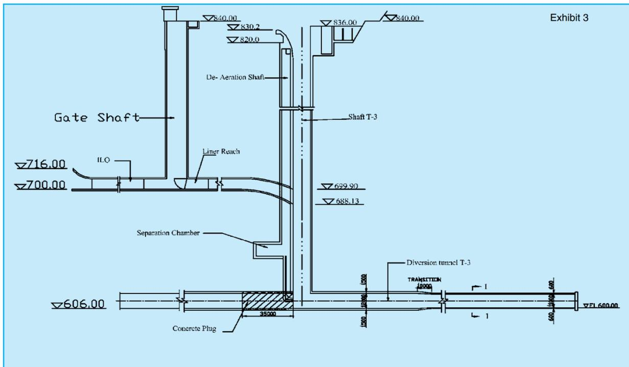
**Right Bank Shaft Spillways and Intermediate level outlet**
