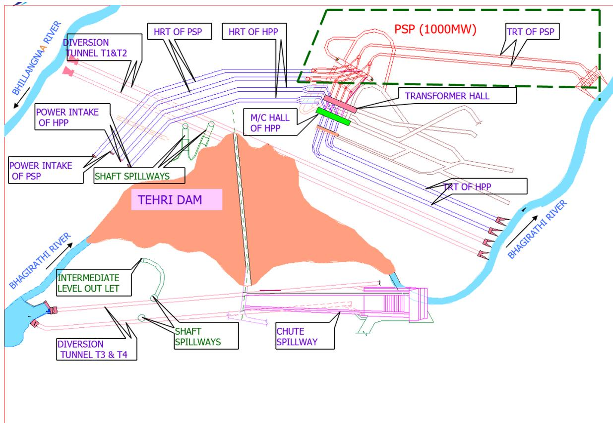
Four head race tunnels of 8.5 m dia. each with intake and an underground power house on the left bank to accommodate four conventional power generating units of 250 MW each (Total installed capacity 1000 MW).
