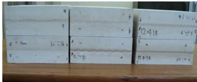
Fig. 60. Samples of unfilled and infilled with asperity angles 0°-0°, 15°-15°, 30°-30°
