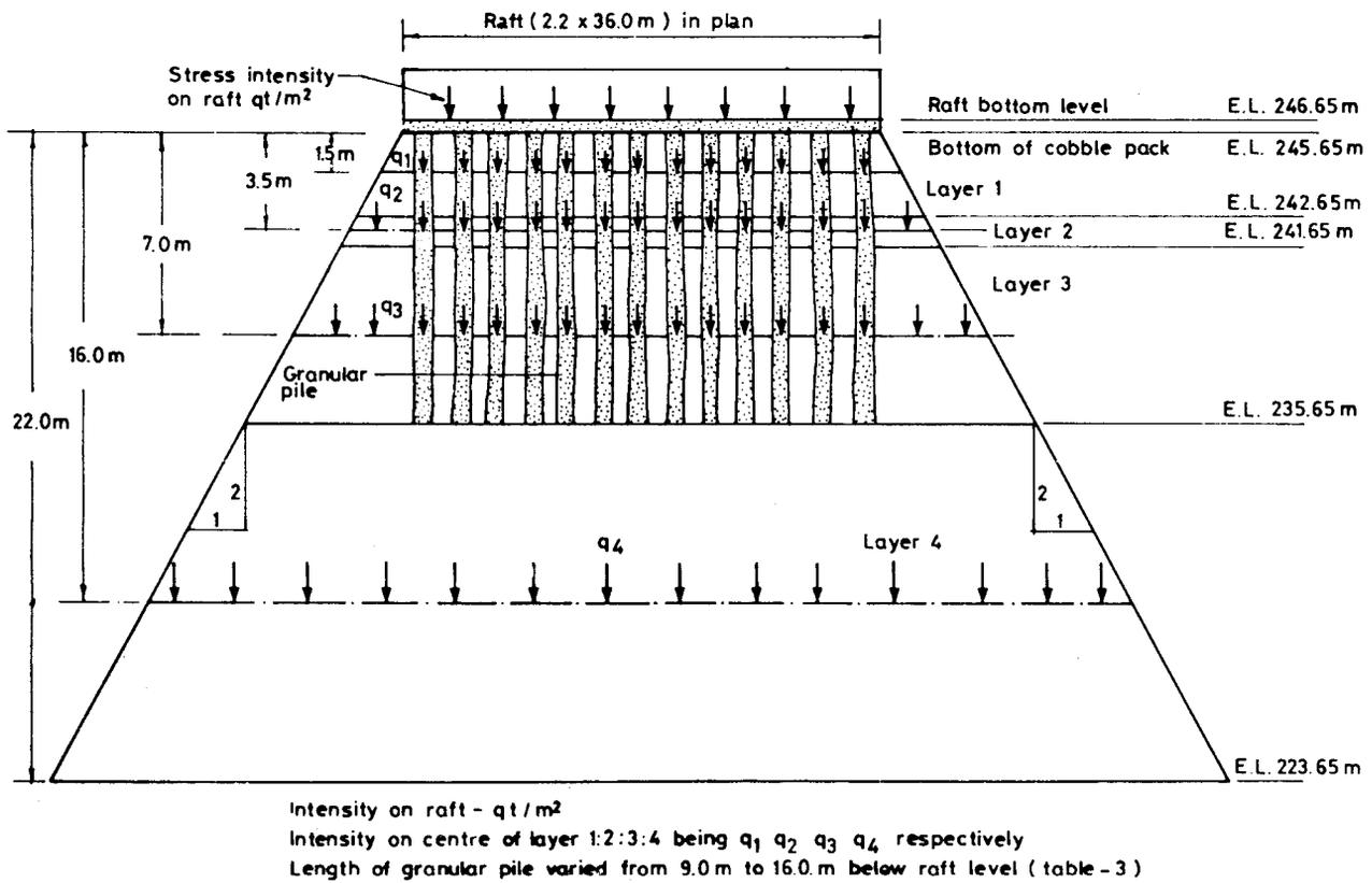
Fig.60 Sub-soil strata for settlement computations
