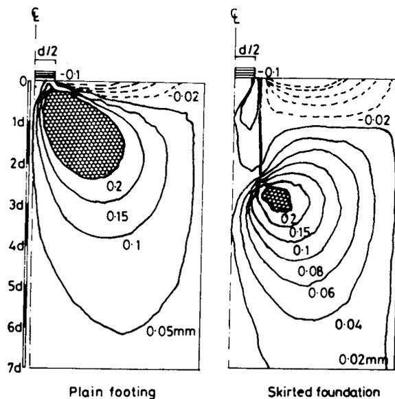
Fig.11 LATERAL DISPLACEMENT OF CONTOUR
