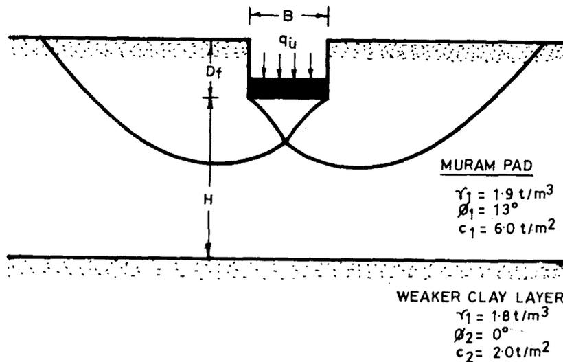
**Fig.31 CONTINUOUS ROUGH FOUNDATION LAYERED SOIL H/B IS LARGE**
