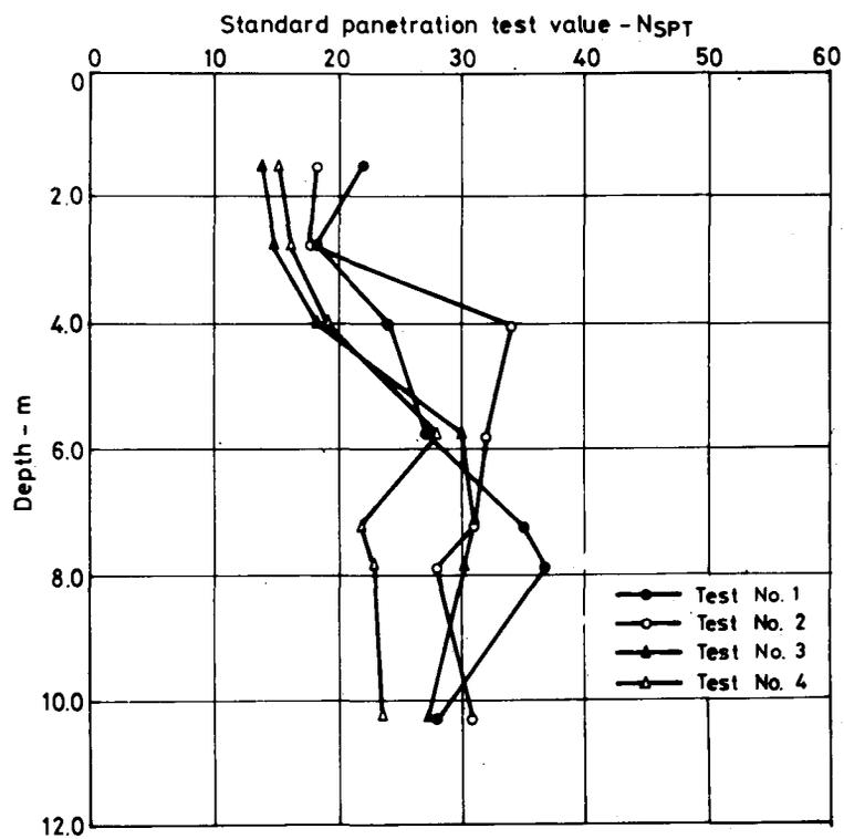
Fig. 56(b) Standard penetration test value vs depth
