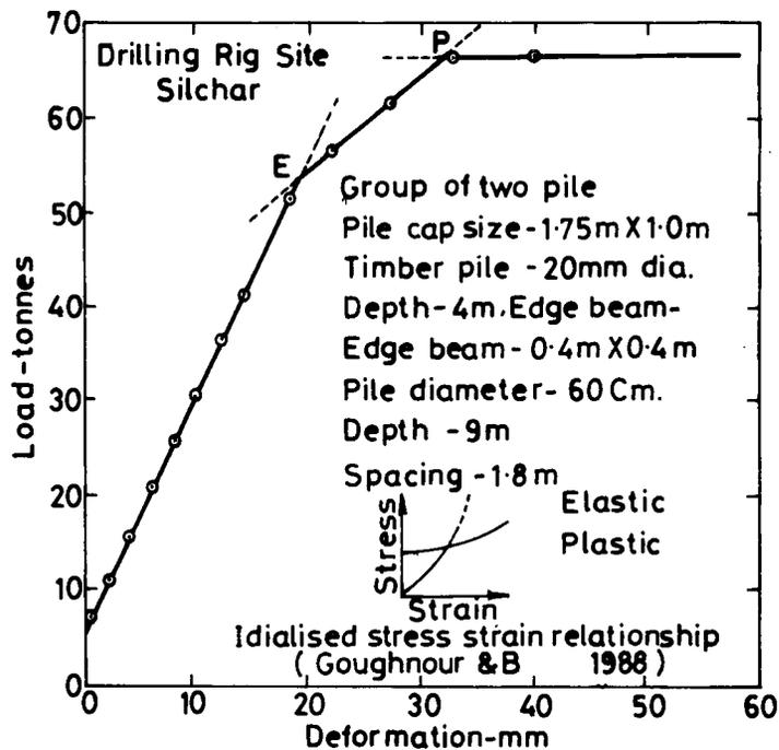
Fig.16 LOAD DEFORMATION BEHAVIOUR OF TWO GRANULAR PILE GROUP WITH TIMBER PILE SKIRTING ( Rao & Ranjan 1988 )
