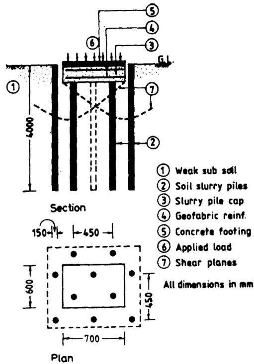
Fig 83 Influence of reinforcing the weak soil immediately below & around the footing by soil slurry piles
