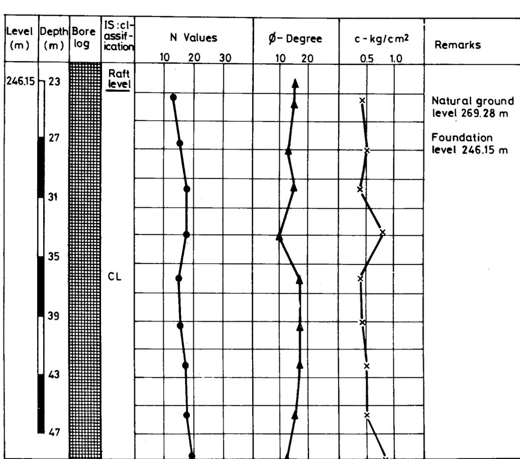
Fig.54(a) Bore log & sub-soil characteristics from, bore hole - 1
