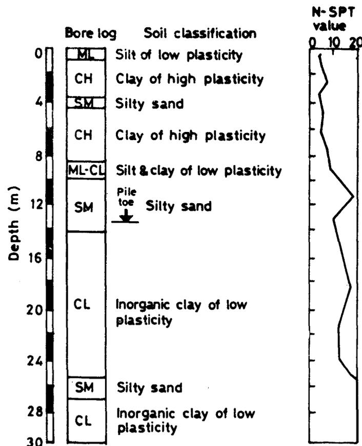
Fig 64. Details of sub soil , bore log and N-SPT values
