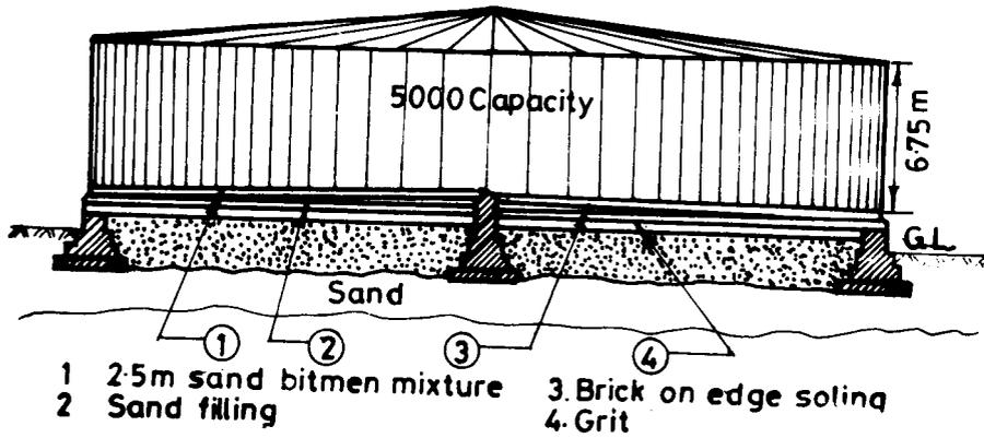
**Fig. 73** Distressed Tank Showing Foundation Details
