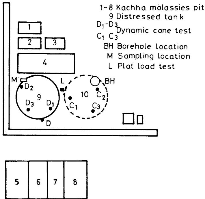
**Fig 72** Site Plan Showing Location of Distressed Tank & Test Points
