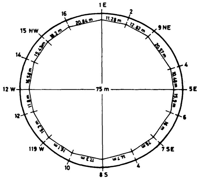
Fig 69 Level points on ring beam (MCO-108)
