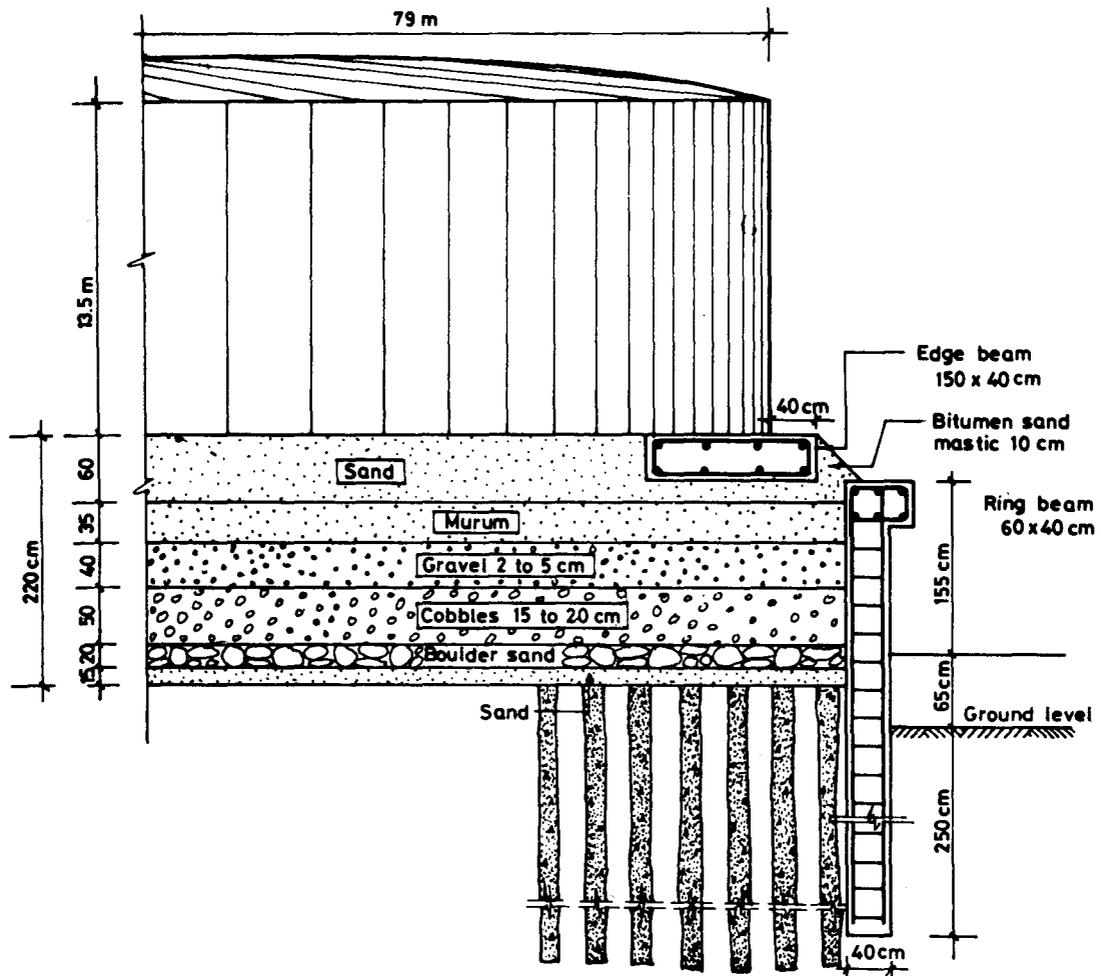
Fig 68 Detail of flexible pad skirt edge beam ring beam etc.
