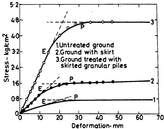
Fig.14 STRESS DEFORMATION BEHAVIOUR OF GROUND TREATED WITH GRANULAR PILES (Rao 1982, Rao & Ranjan 1985)
