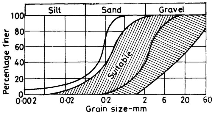
Fig.4 GRAIN SIZE AREA SUITABLE FOR VIBROFLUTATION (Brown 1979)
