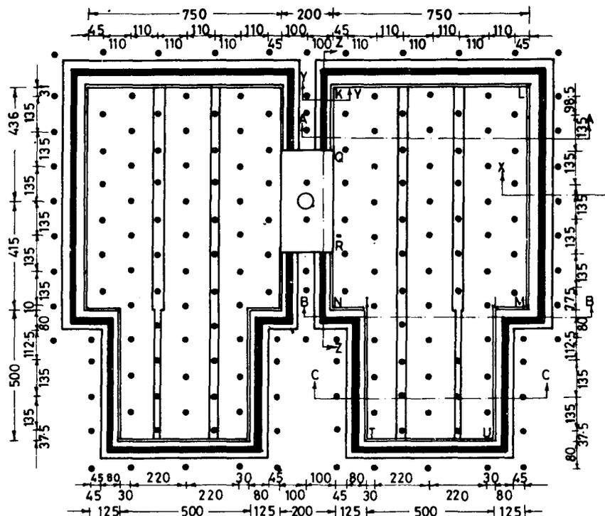
Fig.43 FOUNDATION PLAN SHOWING POSITION OF GRANULAR PILES AND THE SKIRT
