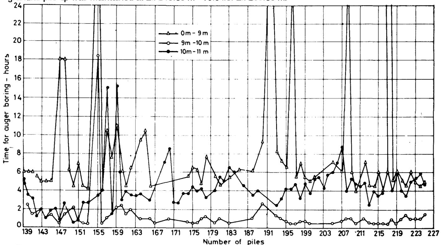
Fig. 63 Time required for installation of piles / bore hole for different depths
