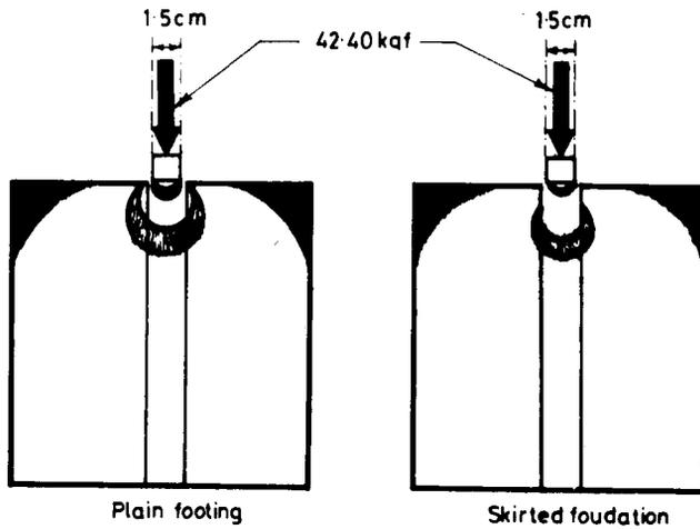
Fig.12 ISOCHROMATICS OF PHOTO ELASTIC METHOD
