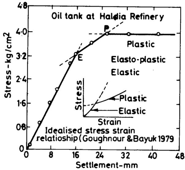
Fig.15 STRESS DEFORMATION BEHAVIOUR OF COMPOSITE GROUND(SOFT CLAY DEPOSIT TREATED WITH GRANULAR PILES )
