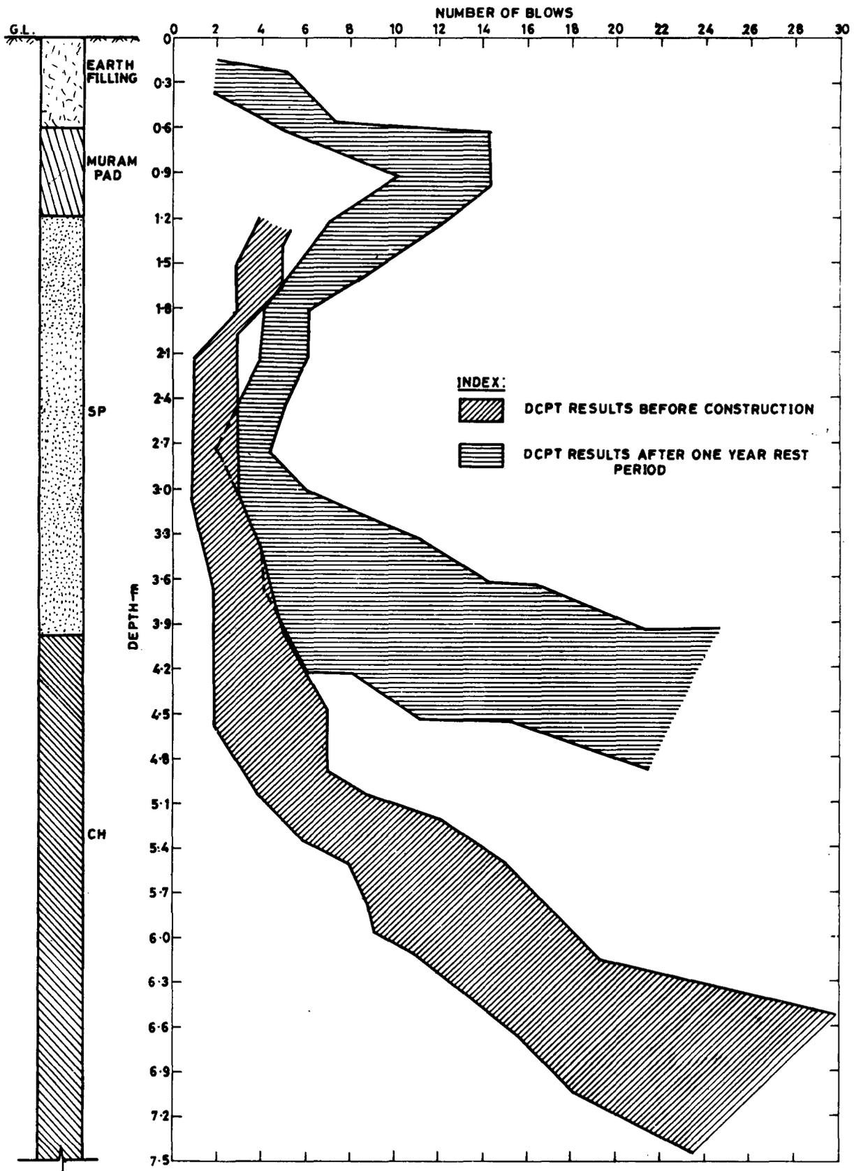
FIG. 37 : DYNAMIC CONE PENETRATION TEST RESULTS BEFORE CONSTRUCTION AND AFTER ONE YEAR OF CONSTRUCTION
