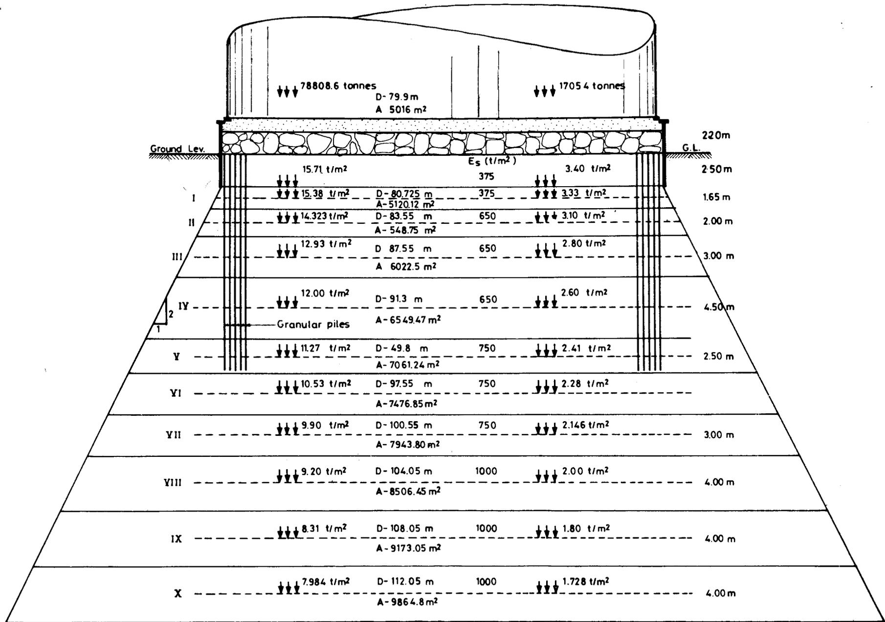
Fig 66 Computation of settlement of composite soil strata supporting mandatory crude-oil steel tank
