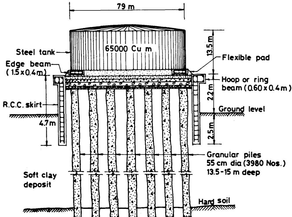
Fig. 65 Mandatory crude oil tank foundation
