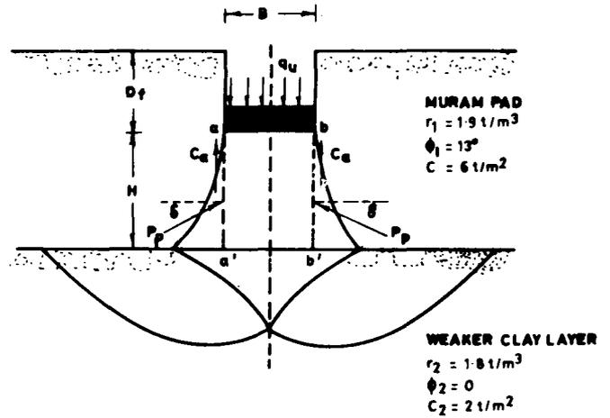
FIG.30 SHALLOW ROUGH COLUMN FOUNDATION ON LAYERED SOIL
