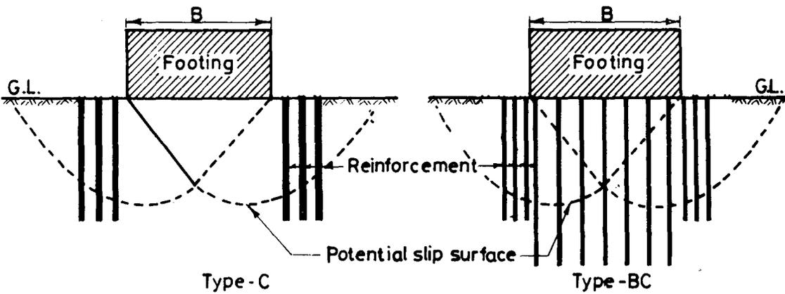
Fig.7 OPTIONS FOR GROUND REINFORCEMENT METHODS
