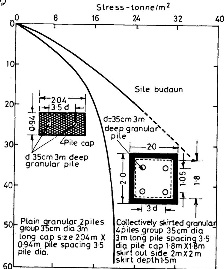
Fig 79 Behaviour of Plain / Skirted Granular Piles Under Load
