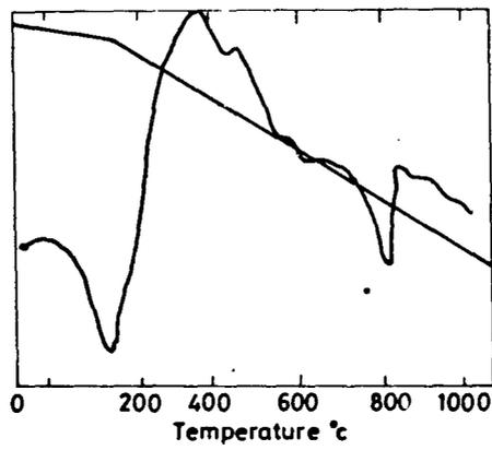
**Fig 77 Differential Thermogram Concrete**
