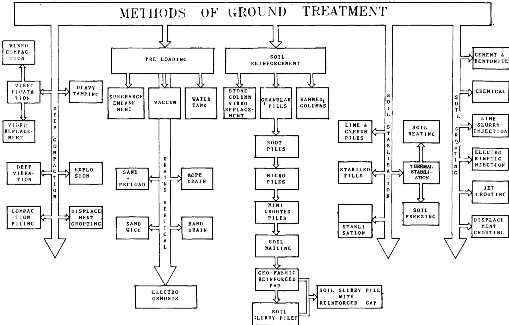
FIG. 2 GROUND TREATMENT METHODS
