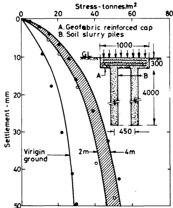
Fig 82 INFLUENCE OF DEPTH OF REINFORCEMENT ON STRESS/DEFORMATION BEHAVIOUR OF COMPOSITE GROUND
