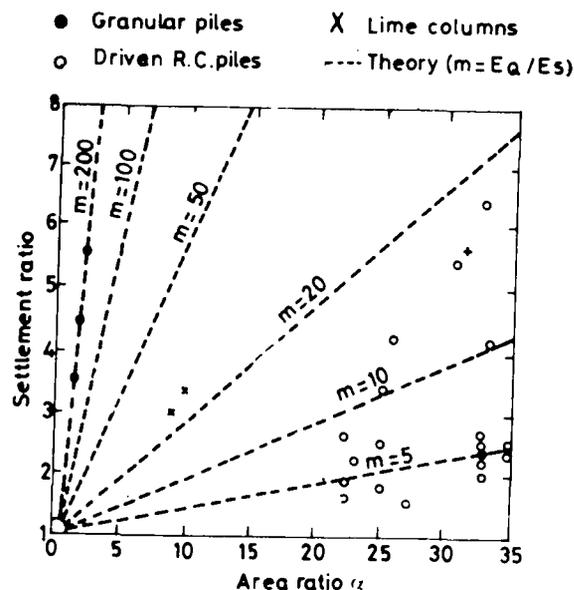
Fig.17 RELATIONSHIP BETWEEN SETTLEMENT RATIO AREA RATIO & EFFECTIVE MODULAR RATIO (Meyerhof 1984)
