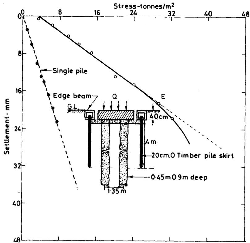
Fig. 50 STRESS-DEFORMATION BEHAVIOUR OF TWO GRANULAR PILE GROUP USING TIMBER PILE SKIRTING
