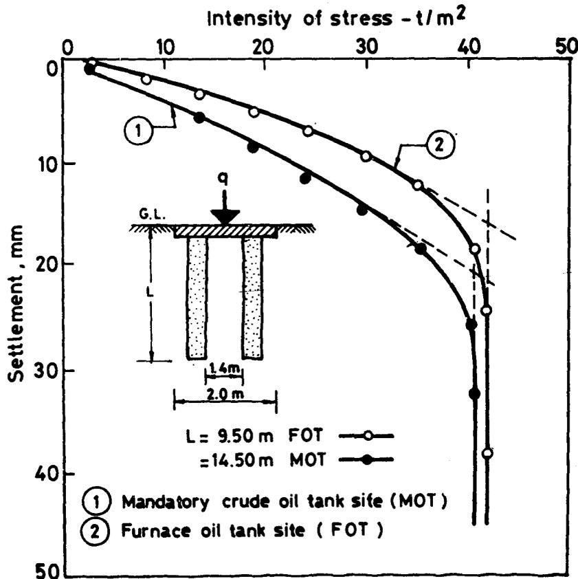
Fig. 67 Stress - settlement curve on composite ground reinforced with group of two granular piles in soft clay deposit
