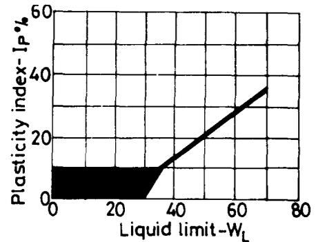
Fig.5 APPLICABILITY OF HEAVY TAMPING IN THE CASE OF CO-HESIVE SOIL
