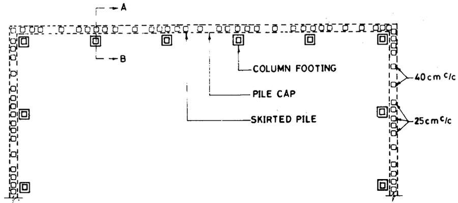
FIG. 39(a): PLAN SHOWING THE LAY-OUT OF R.C.C. SKIRT
