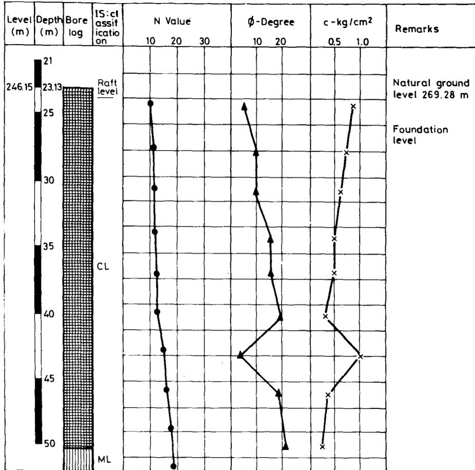
Fig. 54(b) Bore log & sub-soil characteristics from bore hole-2
