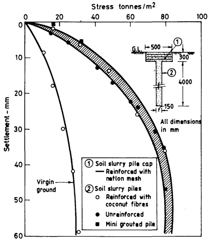
Fig. 81 Stress-deformation behaviour of soil slurry piles with geofabric reinforced pile cap & minigouted pile
