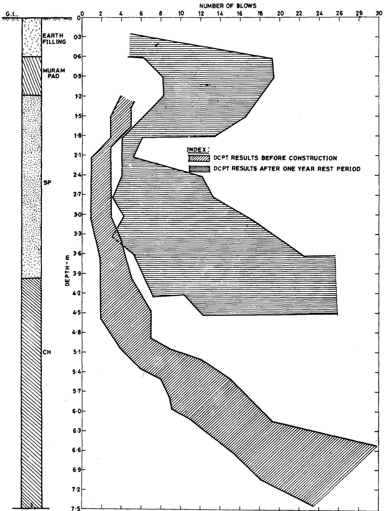
FIG. 38: DYNAMIC CONE PENETRATION TEST RESULTS BEFORE CONSTRUCTION AND AFTER ONE YEAR OF CONSTRUCTION
