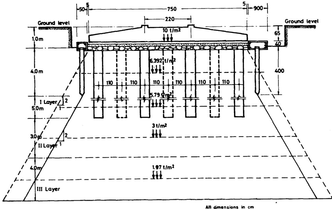
Fig.51 Computation of settlement of skirted granular pile foundation
