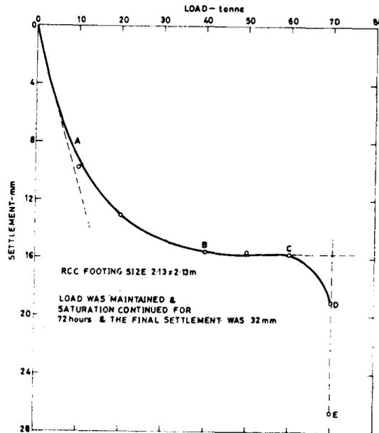
FIG 28 LOAD SETTLEMENT CURVE 2.13x2.13m CONCRETE FOOTING
