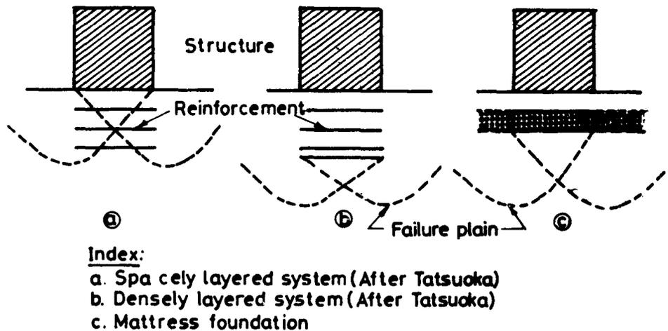
Fig.9 GROUND TREATMENT FOR SHALLOW FOUNDATION
