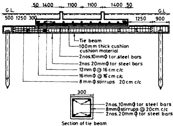
Fig.47 DETAILS SHOWING TIE BEAM
