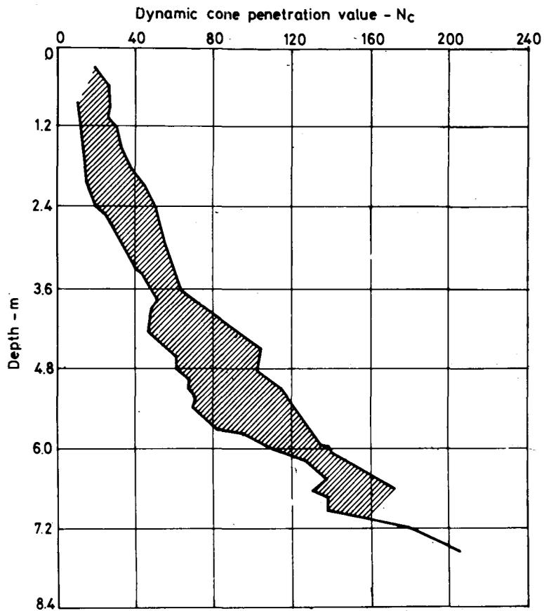
Fig. 56(a) Dynamic cone penetration test value vs depth (Gep-gr - 208 C)
