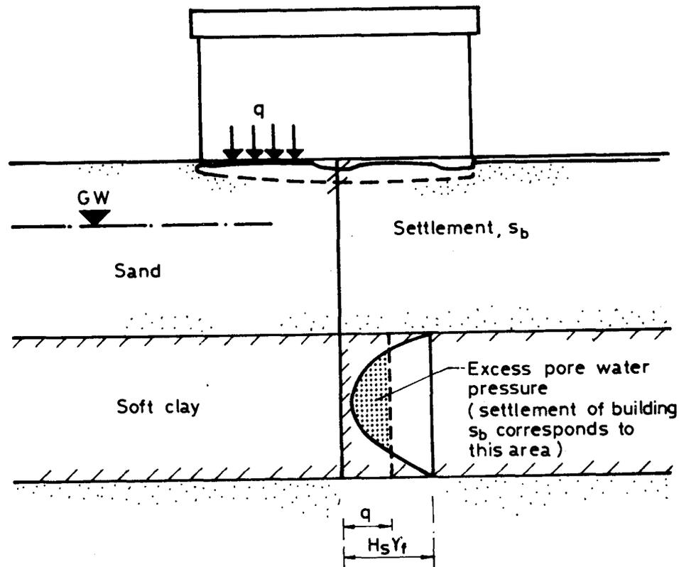
Fig.32 Settlements after preloading
