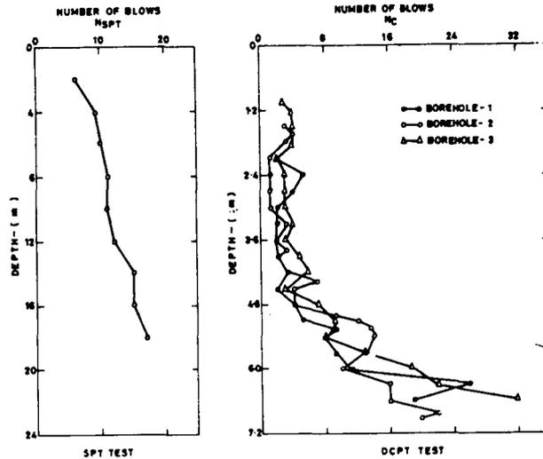
FIG. 26: SPT & DCPT TEST DATA
