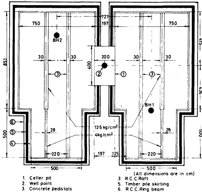
Fig.40 LOADING PLAN
