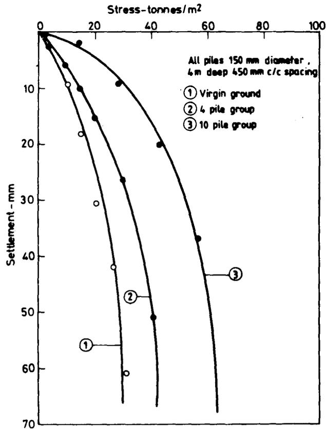
Fig 84 Stress deformation behaviour of weak soil treated with groups of self setting soil slurry piles
