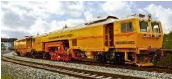
Fig. RW-29(a): Dynamic Tamping Express machine
