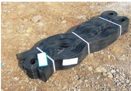
Fig. GC-1(a): Geocells brought folded to site for ease in packaging and transportation
