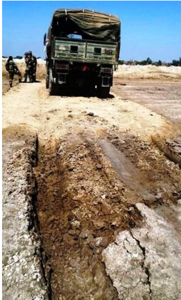
Fig. PV-7©: Comparison between the unreinforced, unpaved pathway (lower portion of the picture) and reinforced, unpaved pathway (upper portion of the picture)
