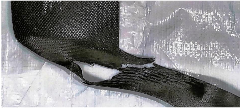
Fig. AP-2: Typical shear failure of strap
