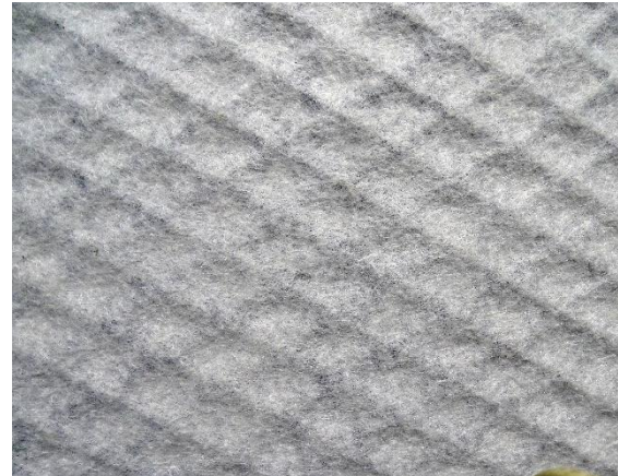
Fig DR-1(b): StrataDrain™ geonet; note the impression of the core within (courtesy Strata Geosystems)
