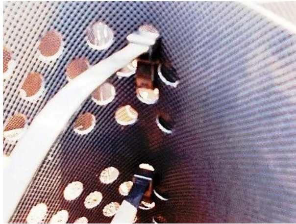
Fig. LF-24(d): Two adjacent panels of StrataWeb® connected together with cable ties
