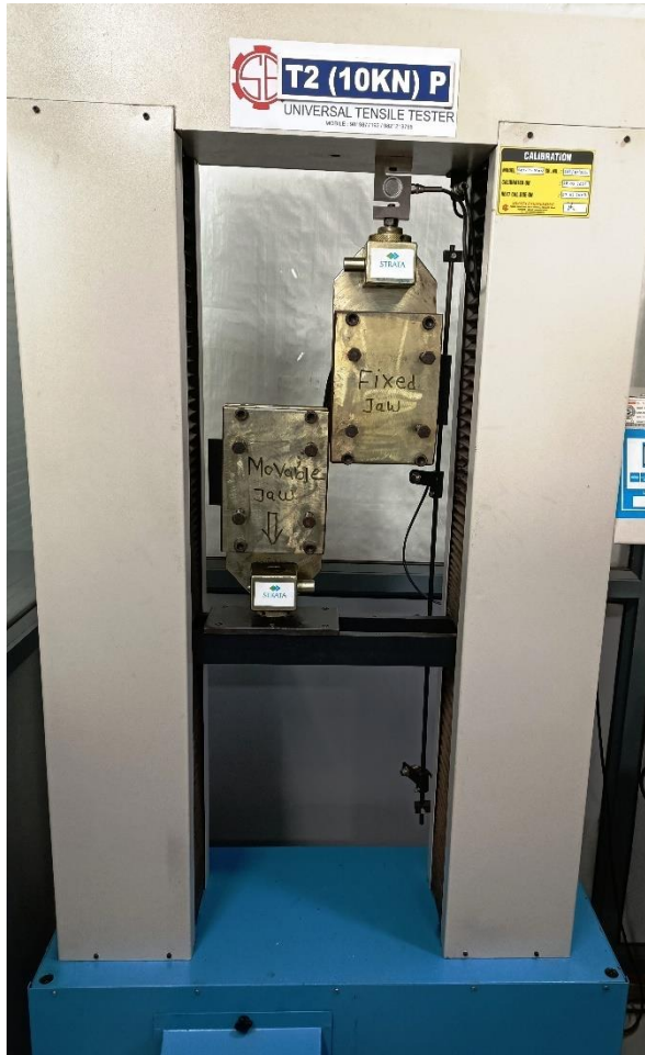
Fig. AP-1(a): The apparatus in shear test mode
