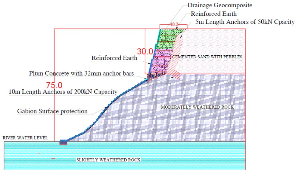
Fig. 5 Slope Stabilization Adopted
